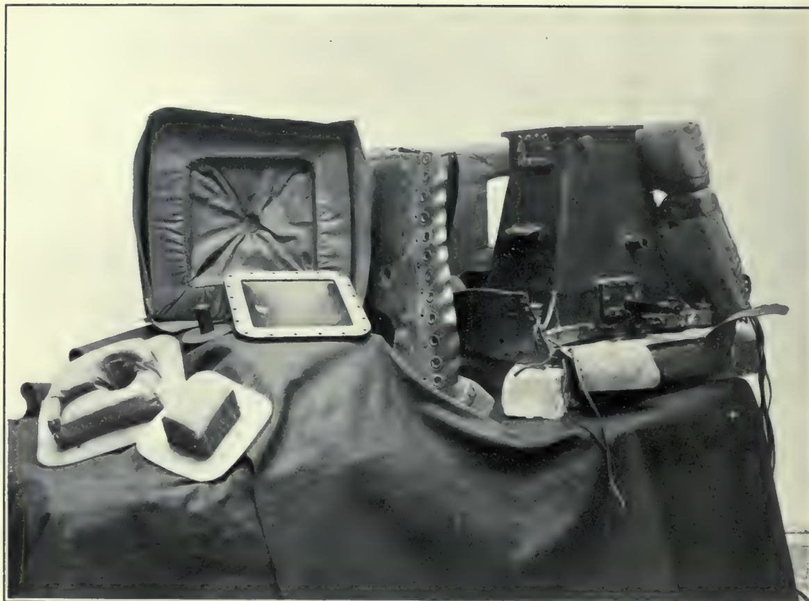
FIG. 4.—FELT-AND-LEATHER CASE FOR TEMPERATURE CONTROL PARTLY REMOVED FROM PENDULUM RECEIVER.
